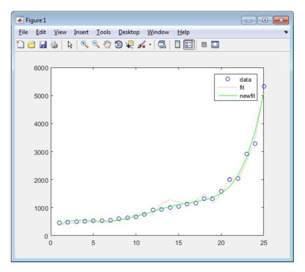
Since the data is closely correlated, but not exactly linearly dependent, the fit curve (dashed line) shows a close, but not exact, fit. The fifth-degree polynomial curve newfit is a more accurate mathematical model for the data.
